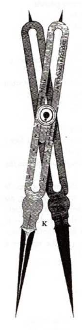
Figura 6: proportional compass [Barrow, 1792].
